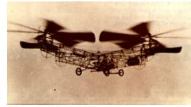
The Flying Octopus accomplished all of its initial test objectives. In 1923, it carried increasingly heavier payloads and set an endurance record of two minutes and forty-five seconds. Nevertheless, the project was canceled when structural changes specified by the Army Air Service produced no substantial improvements in the aircraft's performance.
